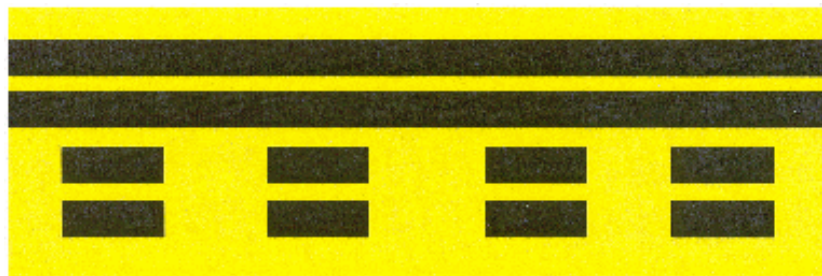
Runway Safety Area/OFZ and Runway Approach Boundary Symbol
